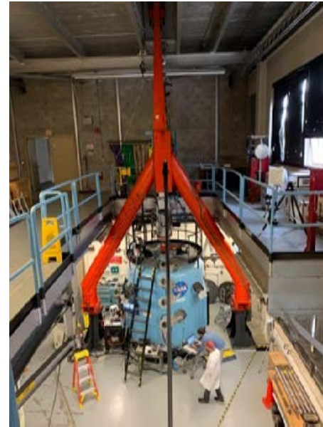
Figure 4. Presents a photo of the AVGR facility, the blue structure is the vacuum chamber, the orange structure raises and lowers the gun. (Photo credit NRL/A. Nicholas).
